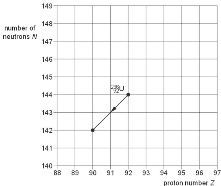
The  $\alpha$ -decay of Uranium-236 ( ${}^{236}_{92}\text{U}$ ) is represented on the grid. This decay produces a nucleus of thorium (Th).
